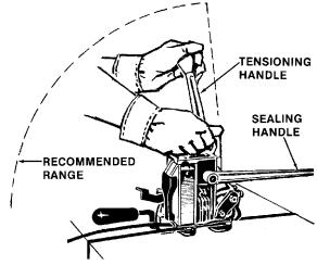
4. Complete the sealing and cut off action by pulling the sealing handle to its full rear position.
