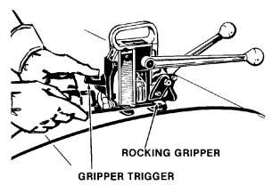
2. Insert the top strap under the feedwheel and insert it sideways into the slot of the strap latch. Pull the excess slack from the strap.
