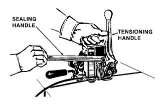
5. To remove the tool from the tensioned strap, return both the tensioning and sealing handles to their forward positions. Place your left hand on the tensioning handle and your right hand on HANDLE the knob. Swing the rear of the tool to your left until it is free of the strap. Inspect the joint to make sure the tool has properly notched the seal.
