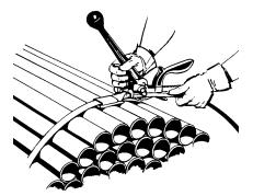
3. While standing to one side of the strap line, apply final tension to the strap.
