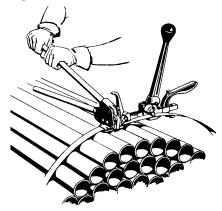
5. Break the strap off over the end of the seal with the nose of the stretcher. Repeat the bending motion if necessary. Do not release tension before break-off and do not tip the stretcher beyond a straight up and down position.
