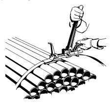
4. Fully notch the seal. If using a single notch sealer, be sure to complete the sealing operation twice on seals requiring two notches.
