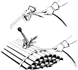
2. Squeeze the two handles as shown. This will open the gripper to allow the upper strap to be inserted through the slotted nose and under the gripper. Pull strap with your left hand to remove slack.
