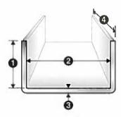
Paper widths of up to 18 inches can be formed into virtually any combination of base sizes, leg sizes and leg lengths, including asymmetrical combinations.
